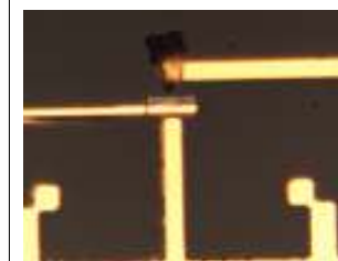
Figure 6. Optical microscope picture of a finished top-gated CNT-FET using TiO 2 dielectric on quartz substrate.
