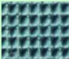
Fig. 1. Square holes etched in a Si wafer
