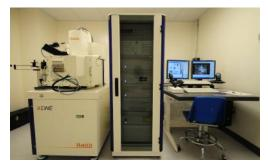
Several key tools for nanofabrication have been acquired in the past few years, including a Raith eLine 150 electron beam lithography system, an Atomate nanowire growth system, and a Beneq atomic layer deposition system.
