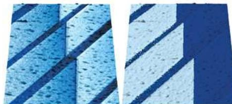
**Figure 6.2.:** PFM amplitude overlaid on AFM topography (left) and PFM phase overlaid on topography (right) on (100) oriented BaTiO<sub>3</sub> single crystal (from Cstech Crystals). The amplitude and phase image show 90° and 180° domain walls in BaTiO<sub>3</sub>. (10  $\mu\text{m}$  scan courtesy of V. R. Aravind, K. Seal, S. Kalinin, ORNL, and V. Gopalan, Pennsylvania State University.)
