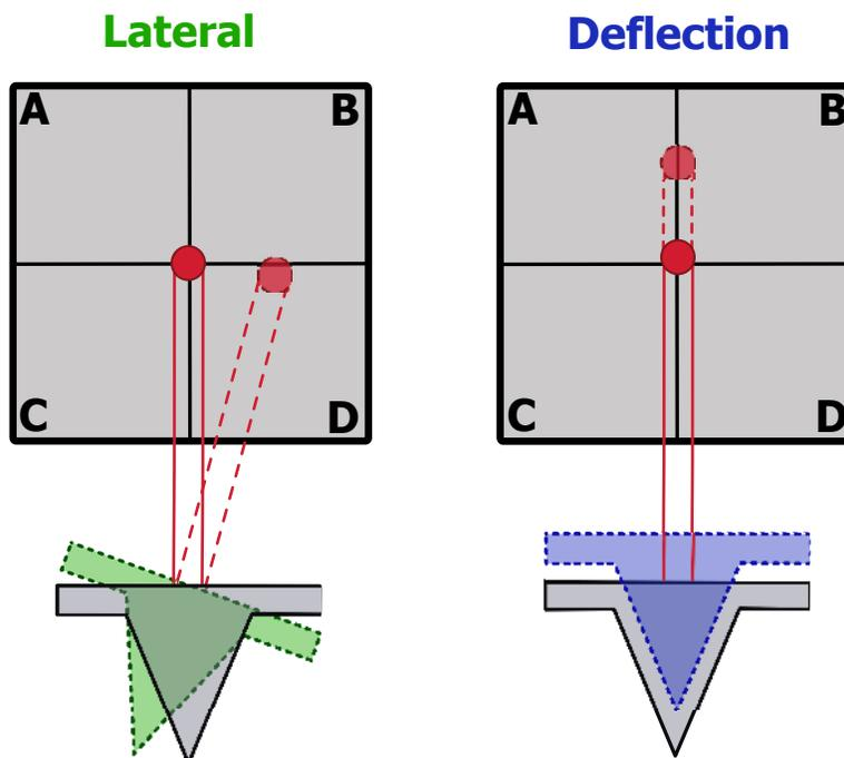
Figure 3.1.: The Lateral signal versus the Deflection signal on the photodetector.
