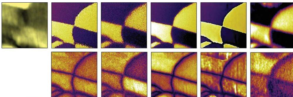
**Figure 6.27.:** High Frequency PFM using Asylum’s fast photodiode on a ceramic PZT sample at different frequencies (phase left, amplitude right) – below first resonance (top row) and at cantilever resonances (all others) using a MikroMasch NSC 35B cantilever. 1 $\mu$ m scans. (Image courtesy of K. Seal, S. Kalinin, S. Jesse, and B. Rodriguez, Center for Nanophase Materials Science, ORNL.)
