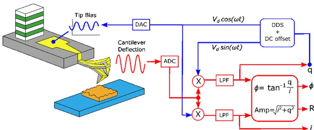
**Figure 11.1.:** Schematic showing how SKPM is performed on Asylum Research AFMs. The probe tip is driven electrically with an AC bias. The potential difference between the tip and the sample causes the probe to mechanically oscillate. These mechanical oscillations are then negated by a feedback loop on the bias. The voltage required to negate the oscillations (i.e., match the probe to the sample) is captured and recorded as the surface potential channel in the AFM software.
