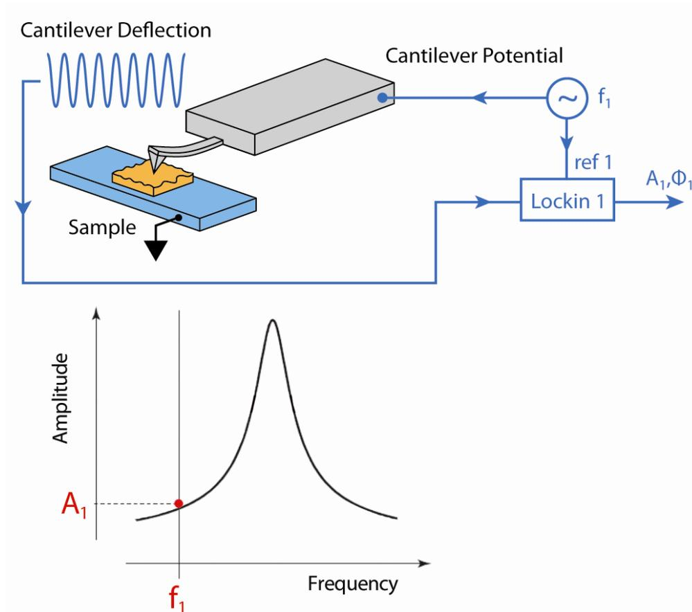
Figure 7.1.: A diagram of Single Frequency PFM
