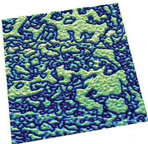
**Figure 6.29.:** (001) domains in a PZT thin film, 3.8 $\mu\text{m}$  scan. (Image courtesy N. Polomoff and B. D. Huey, University of Connecticut Institute of Materials Science. Sample courtesy R. Ramesh, UC Berkeley.)
