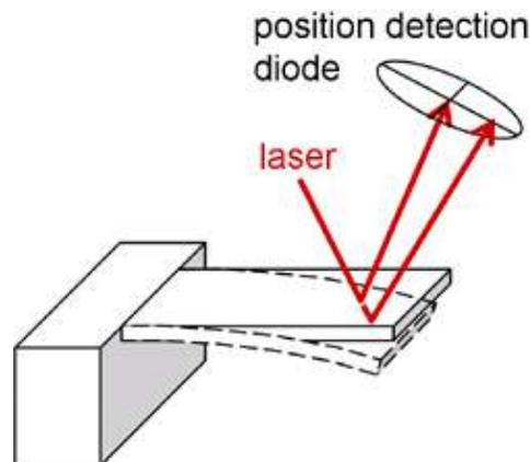
Figure 22.2.: Cantilever optical detection. The optical lever.
