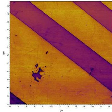
3. A common problem is the loading force being too small. If you have tried adjusting the drive voltage and still do not see good domain contrast, try increasing the loading force. Click 'Stop' and decrease the deflection with the PD knob (or PD motors on Cypher), then retune on the surface. The contact resonance changes depending on the loading force.
