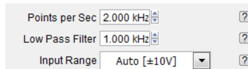
**Note** You can set the digital filter to as low as needed; however, below 50Hz, artifacts may appear. Ensure that your filter value is set to at least twice the frequency of your function wave. More complex wave forms (non-sinusoidal) require much higher bandwidths to drive and acquire.
