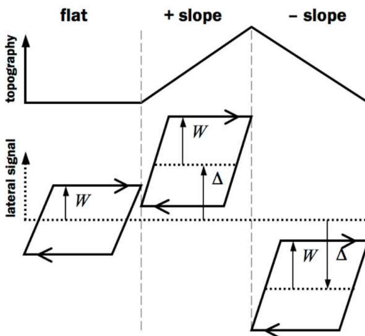
**Figure 3.4.:** Friction loops on flat, inclined, and declined surfaces at a given applied load. The half-width ( $W$ ), representing the frictional response, only slightly varies; while the offset ( $\Delta$ ), due to the surface tilt, varies substantially. The load dependence of  $W$  and  $\Delta$  are used to determine the lateral force sensitivity of the cantilever.
