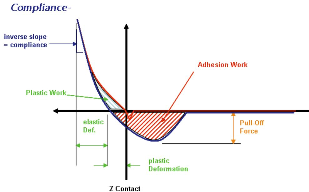
Figure 18.3.: Compliance force spectroscopy classification. Pushing can measure compliance forces.
