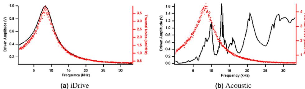
**Figure 16.5.:** Cantilever tunes acquired with iDrive AC mode (left) and piezo-driven (acoustic) AC mode (right) showing both the mechanical response (black curves) and the thermal noise power spectrum (red curves).
