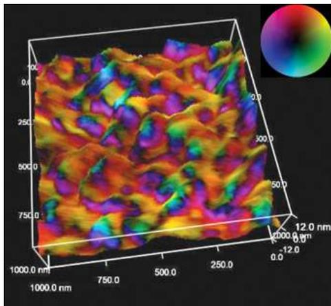
**Figure 6.6.:** BST film with vector PFM overlaid on AFM topography, 1 $\mu$ m scan. (Image courtesy of C. Weiss and P. Alpay, Univ. of Conn., and O. Leaffer, J. Spanier, and S. Nonnenmann, Drexel University.) Color wheel indicates PFM vector orientation.
