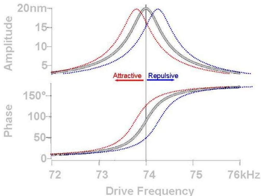
**Figure 5.6.:** A shift in resonance frequency,  $f_o$  (at constant amplitude) as the tip interacts with surface results in phase shift of the AC signal: Decrease in  $f_o$  results in phase increase (attractive mode), while increase in  $f_o$  results in phase decrease (repulsive mode). The colors represent the color of the phase on the Sum and Deflection Meter Panel.
