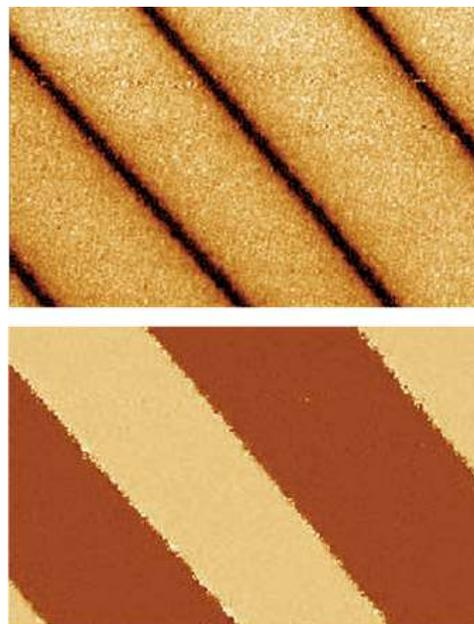
**Figure 6.30.:** PPLN amplitude (top) and phase image (bottom) acquired with the MFP NanoIndenter, 50 $\mu\text{m}$  scan.
