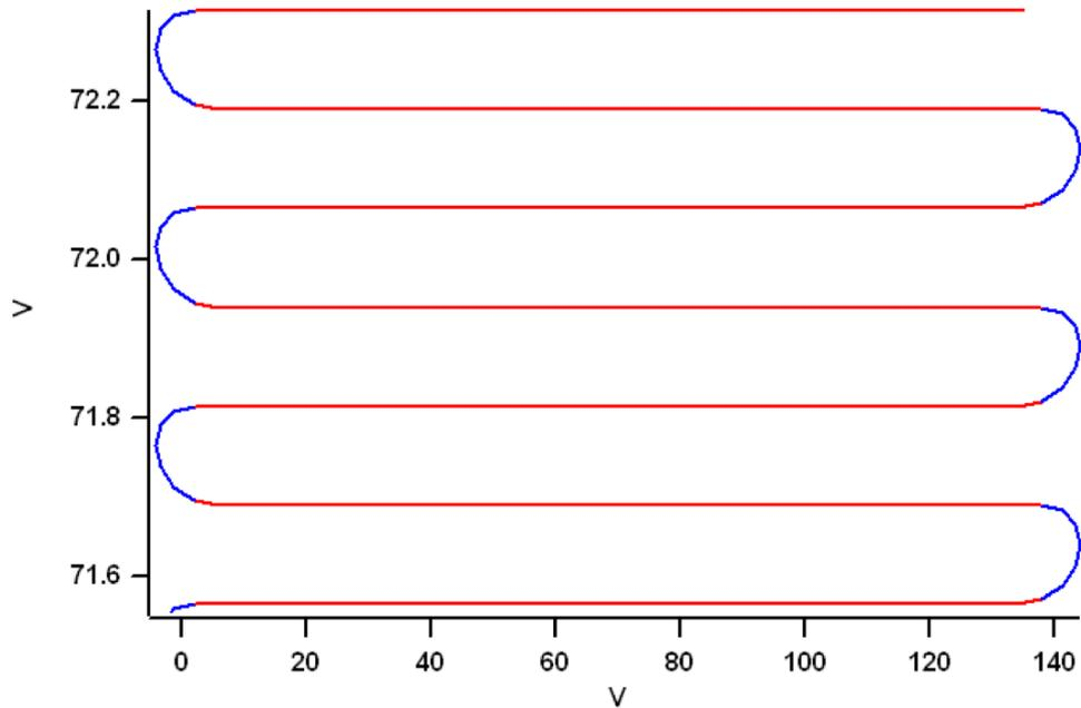
**Figure 23.3.:** Motion of the Tip Across Surface in Ortho Imaging. The X-axis is the fast axis drive, while the Y-axis is the slow axis drive. Three scan lines are shown. The blue sections denote turn-around regions.
