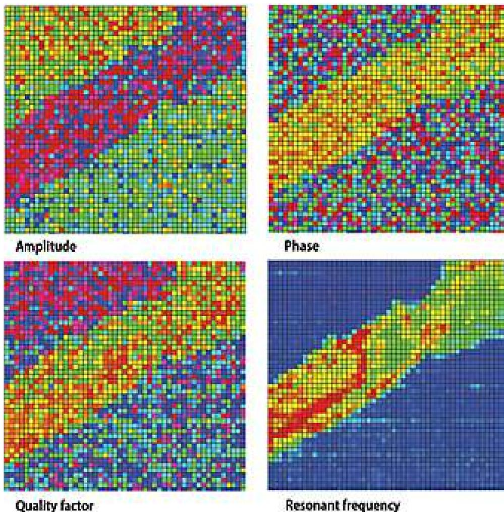
**Figure 6.26.:** Amyloid fibril (bovine insulin) on mica imaged in water using BE-PFM technique, 250nm x 250nm. (Image courtesy of G. L. Thompson, V. V. Reukov, A. A. Vertegel, M. P. Nikiforov, Clemson University, Dept. Bioengineering, and S. Jesse, S. V. Kalinin, Oak Ridge National Lab.)
