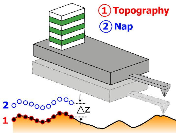
**Figure 10.1.:** During Nap mode, the probe is first scanned across the sample surface, then raised to a delta height defined by the user. This allows for detection of long-range forces between the tip and sample.
