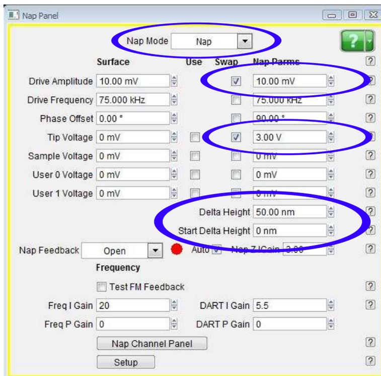
**Figure 12.4.:** Here the Nap Panel is set up for EFM operation. The relevant fields have been circled. The “Use” column in the middle left has check boxes that, when checked, cause that parameter to be used during the main scan. The “Swap” column has check boxes that, when checked, allow those fields to be used during the parm swap/ nap scan.
