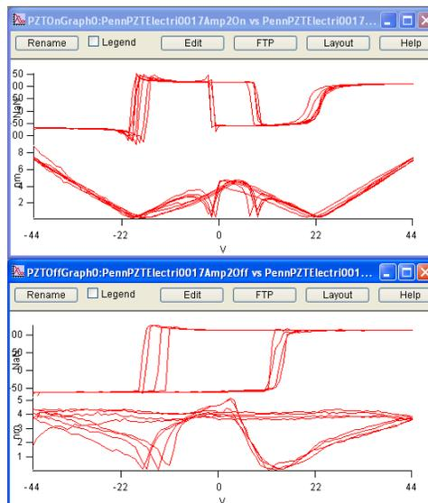
**Figure 8.9.:** The applied (“On”, top graph) and remnant (“Off”, bottom graph) hysteresis loops obtained from the processed time waves of figures 8.7 and 8.8. The phase loops are on the top of each window, and the amplitude “butterfly” loops are on the bottom.
