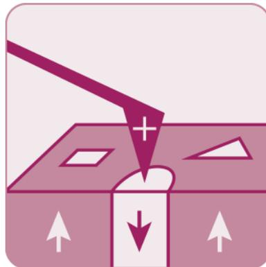
PFM can also be used to modify the ferroelectric polarization of the sample through the application of a bias. When the applied field is greater than the coercive electric field, the field can induce ferroelectric polarization reversal. The MFP3D Lithography PFM mode can be used to write complex patterns by importing a grey scale image that is transformed to a bias map.
