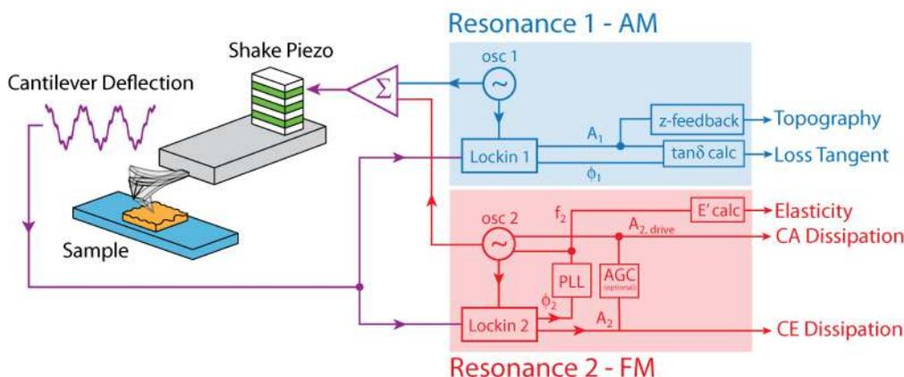
**Figure 15.1.:** AM-FM Mode. The first mode amplitude is controlled to create a topographic image of the sample (blue). The second mode is used to calculate elasticity and tip-sample stiffness (red).
