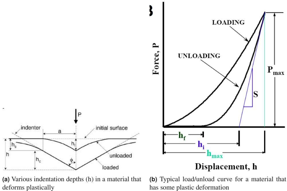
**Figure 18.21.:** Qualitative schematic commonly used in nanoindentation to illustrate the difference between maximum indentation ( $h$ ) and indentation depth after load is removed ( $h_f$ ). (Figure adapted from Oliver, W.C., Pharr, G.M., *J. Mater. Res.* 2004, 19 (1) p3-20.)
