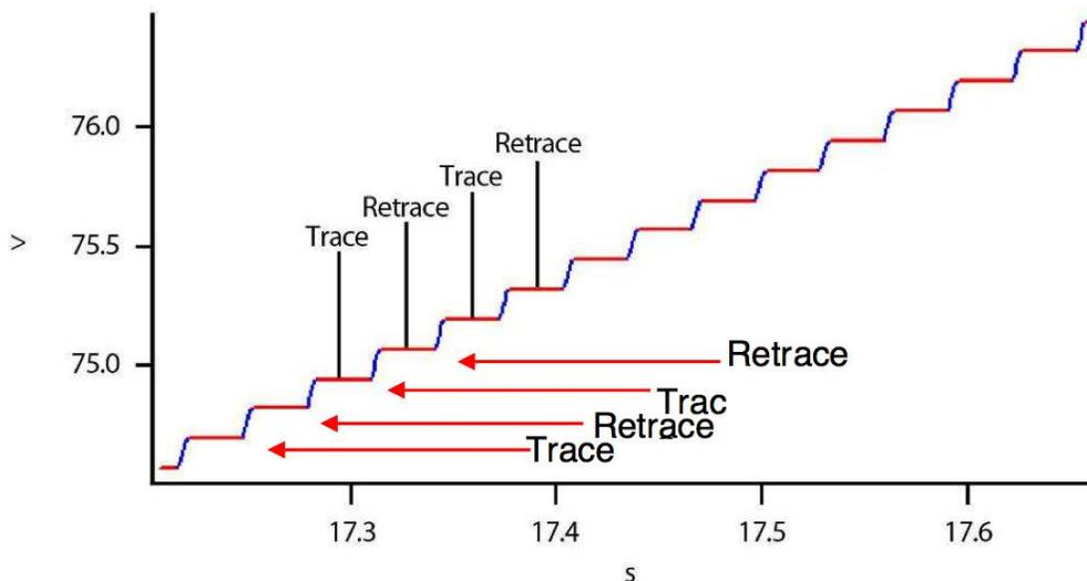
**Figure 23.2.:** Slow Axis of Ortho Scan. In the above image, the vertical axis is Y piezo voltage (scan angle  $0^\circ$ ); horizontal axis is time. Axis limits are zoomed in to show the same region as in preceding Figure (Slow Axis of Raster Scan). The blue sections denote turn-around regions. Approximately seven scan lines are shown here, each comprising two steps (one for Trace and one for Retrace).
