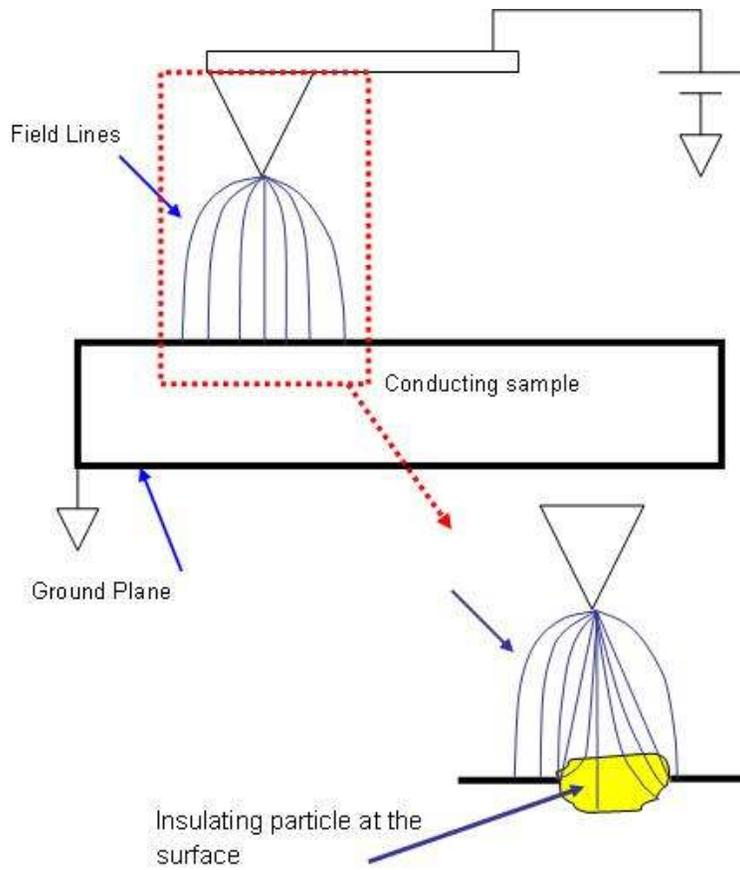
**Figure 12.2.:** Effects of introducing an insulator into a metal sample. EFM is generally not suitable for this sample configuration, as the field lines show little shift. Any shift would be difficult to discern from the changes in topography.
