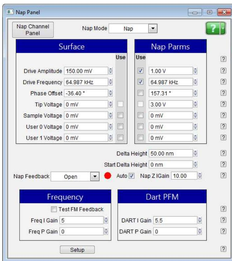
**Figure 10.2.:** Nap Panel, opened from the menu: *AFM Controls > Nap Panel*(Ctrl + 9)
