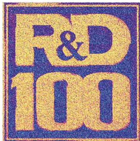
**Figure 6.7.:** R&D 100 logo written on a sol-gel PZT thin film by PFM lithography. PFM phase is overlaid on top of the rendered topography, 25  $\mu$ m scan. Oak Ridge and Asylum Research were awarded an R&D100 award for Band Excitation in 2008.
