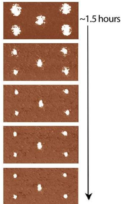
**Figure 6.24.:** Stable imaging using DART allows relaxation studies. This series of images shows the relaxation of sol-gel taken at different intervals for approximately 1.5 hours. 3.5  $\mu\text{m}$  scan.
