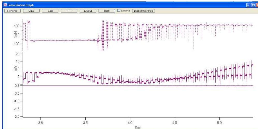
**Figure 8.8.:** Zoomed in region from Figure RawData . Here, the individual steps from the stepped SS-PFM method of<sup>8</sup> are evident. Repeat the above steps as many times as you want, adjusting the drive parameters accordingly. If you notice noise during the higher voltage portions of the curves, you may have your *Freq Igain* set too large. Reduce it until the effect disappears.
