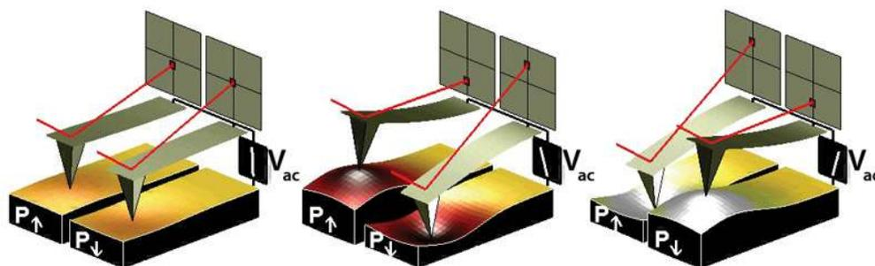
**Figure 6.4.:** Sign dependence of the sample strain. When the domains have a vertical polarization that is pointed downwards and a positive voltage is applied to the tip, the sample will locally expand. If the polarization is pointed up, the sample will locally contract. The phase of the measured response is thus proportional to the direction of the domain polarization. (Image courtesy of S. Jesse, ORNL.)
