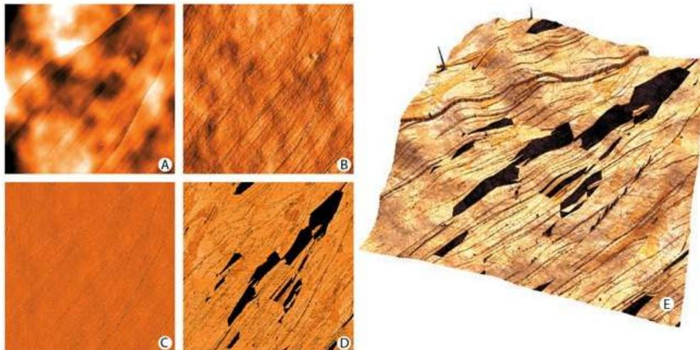
**Figure 14.3.:** 30µm image of a HOPG surface acquired with an Olympus AC240-R3 Silicon cantilever. (A) Height channel, (B) Amplitude 1 channel, (C) Phase 1 channel, (D) Amplitude 2 channel, (E) Phase 2 channel overlaid on 3D rendered Height channel.
