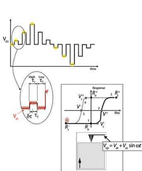
**Figure 6.8.:** Switching spectroscopy PFM diagram (see text for discussion). (Reused with permission from Jesse, Baddorf, and Kalinin, Applied Physics Letters, 88, 062908 (2006). Copyright 2006, American Institute of Physics.)
