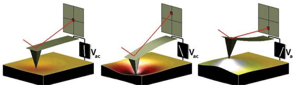
**Figure 6.3.:** Depiction of PFM operation. The sample deforms in response to the applied voltage, which in turn causes the cantilever to deflect, which can then be measured and interpreted in terms of the piezoelectric properties of the sample. (Image courtesy of S. Jesse, ORNL.)
