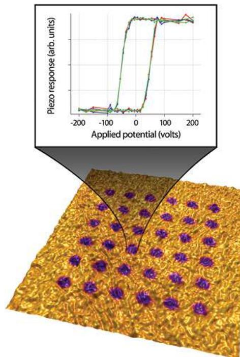
**Figure 6.9.:** Rendered topography of a LiNbO<sub>3</sub> sample with the PFM signal overlaid on top, 4μm scan.
