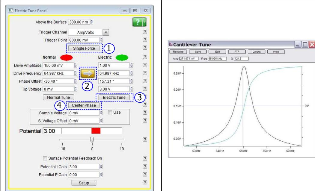
The image shows two software windows. On the left is the 'Electric Tune Panel' with various control fields. On the right is the 'Cantilever Tune' window showing a resonance graph.
