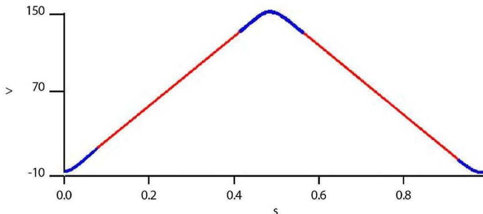
**Figure 23.1.:** Fast Axis X Piezo Drive (at  $0^\circ$  scan angle). Y-axis of graph is piezo voltage; X-axis is time. The rounded caps (blue regions) are called the “turn-around”, where the fast axis changes direction. Data from the turn-around is not typically saved, though it is possible to access it for special applications.
