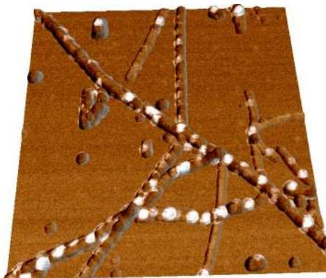
**Figure 16.2.:** Insulin Fibrils imaged in water. Phase signal overlaid onto topography. The “white” regions in the image are from the phase channel and correspond to higher energy dissipation. 1 $\mu$ m scan.
