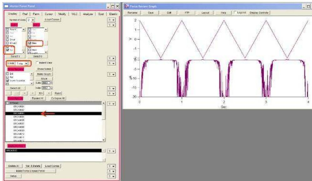
**Figure 9.7.:** Current vs time. It is often useful to display the current vs time, particularly for samples that degrade or improve in conductivity with time. Si will oxidize as more current is passed through it if there is moist air near the surface.
