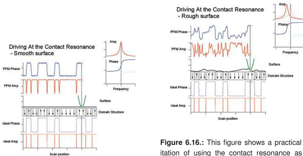
**Figure 6.15.:** This figure shows the same situation as described in Figure 6.14 on page 65, except that here we are using resonance enhancement to boost the small PFM signal. The inset frequency tune in the upper right corner shows the drive frequency. In this case, since the  $Q$ -factor of the resonance is 100, the SNR of the measured PFM amplitude (red, thick curve) and phase (blue, thick curve) has dramatically improved.
