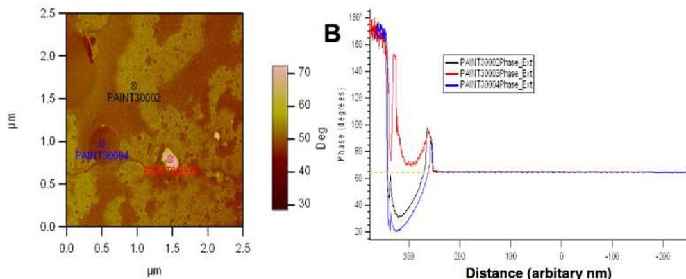
**Figure 18.28.:** AC “point and click” force curves on heterogeneous sample. A) Phase image of paint sample with location of user-defined force curves; B) individual AC force curve Phase vs. distance (Z)—orange dash line indicates Free Air Phase values of  $\sim 64$  degrees. (Yes, that is the di color table on the 3D.)
