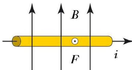
**Figure 16.1.:** The Lorentz Force  $F$  is orthogonal to both current  $i$  and the magnetic field  $B$  and is pointing out of the page.
