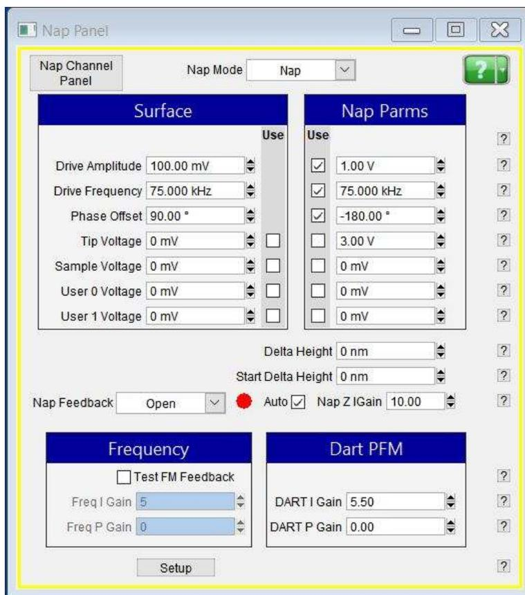
**Figure 11.3.:** Nap Panel configured for SKPM scan. The values in the parameters may vary depending on your tip and sample.
