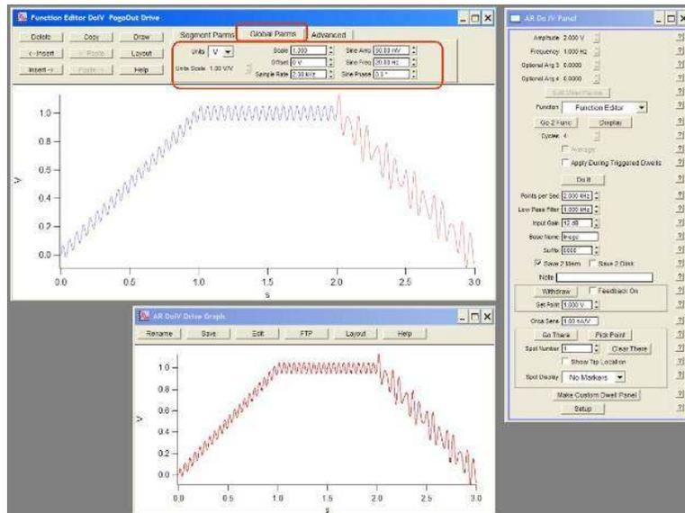
**Figure 9.5.:** Use the Global tab to modify all the individual segments at one time. Of particular use in this section is the *Scale* field. This function allows you to scale up or down the entire wave function you have created. For example, if you had a custom wave from 0-1V with a dwell, scaling it by 5 would make it go from 0 to 5V.
