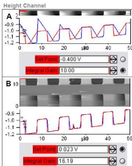
5. The second set of parameters to adjust are the *Scan Rate* and *Scan Angle*. Having a vague idea of the orientation of the tip on the cantilever can make scanning at  $90$  degrees more advantageous than at  $0$  degrees because of the shape of the tip at the end of the cantilever. Some cantilever manufacturers compensate for the slight angle that the cantilever is mounted relative to the surface by having the front and back angles of the pyramid at different angles.
