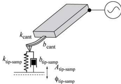
**Figure 6.13.:** In PFM, the cantilever voltage is modulated, usually at some fixed frequency. This causes the sample to distort at some amplitude and phase. Mediated by the contact mechanics, this drives the tip which, in turn, is monitored by the AFM sensor.
