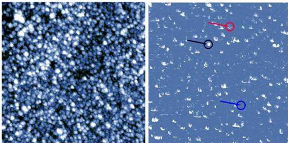
**Figure 9.2.:** Fairly typical thin film CAFM image. Note that tip shape artifacts are visible on the current image (left), but not on the topographic image (right). As the metal coating on the probe tip wears, or if the tip is contaminated, these artifacts will be more prominent. Rocky Mountain Nanotech now makes a solid Pt probe that does not suffer from this problem.
