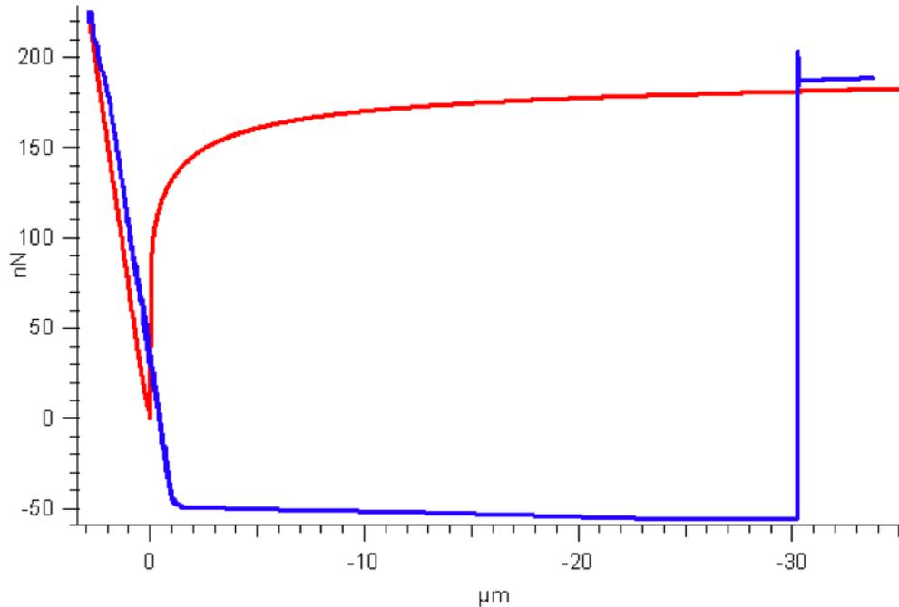
Figure 18.25.: Large surface forces can act on a sphere affixed to cantilever
