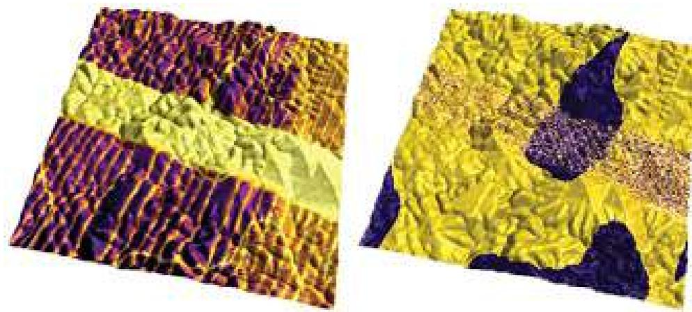
**Figure 6.5.:** Vertical PFM amplitude overlaid on AFM topography (left) and PFM phase overlaid on AFM topography (right) images of lead titanate film, 5  $\mu\text{m}$  scan. (Images courtesy of A. Gruverman and D. Wu, UNL. Sample courtesy H. Funakubo.)
