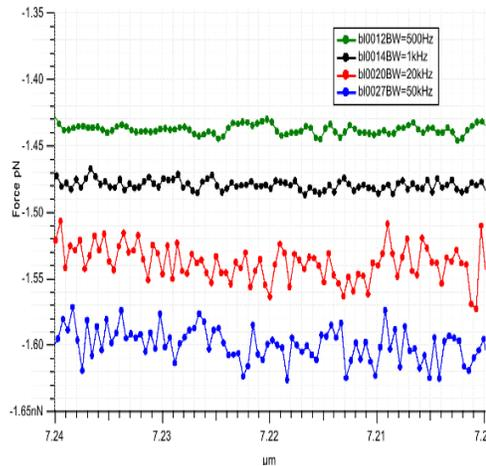
(a) Various data streams from a free air portion of a force curve collected at 2kHz (i.e., 2,000 points/sec) with different low pass filter settings. Notice higher filter settings are noisier.
