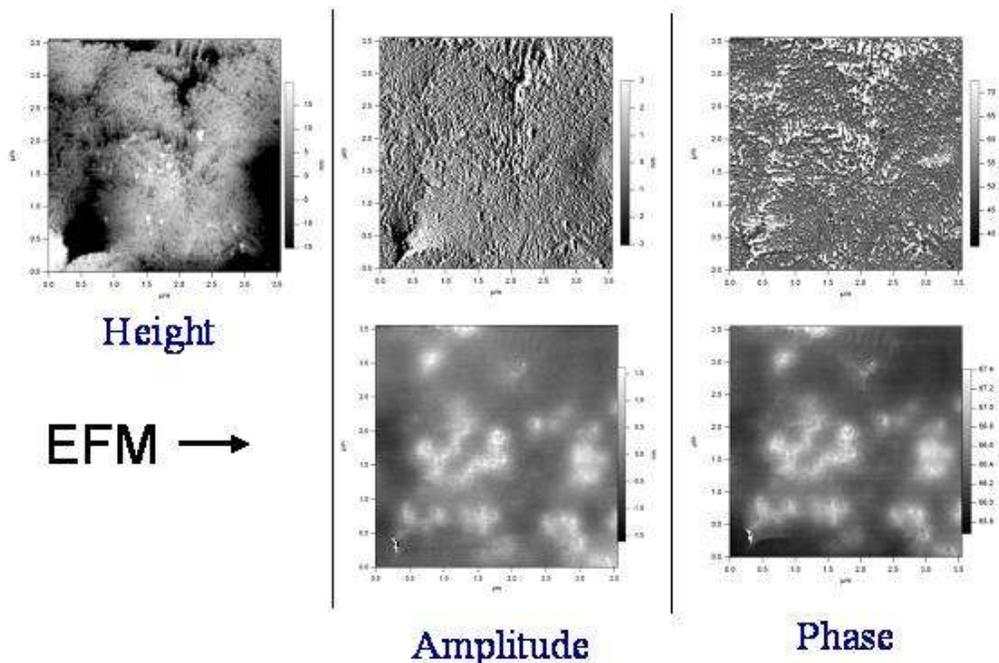
**Figure 12.5.:** EFM image of polypropylene with carbon black particles (CB) imbedded into it. The areas of contrast in amplitude and phase are due to the presence of CB particles either at or below the surface of the polypropylene.
