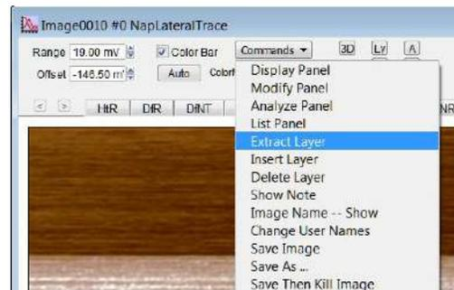
4. In the Igor command line (CTRL+J), subtract the **Nap Lateral Trace** wave from the **Nap Lateral Retrace** wave and divide that result by 2.
