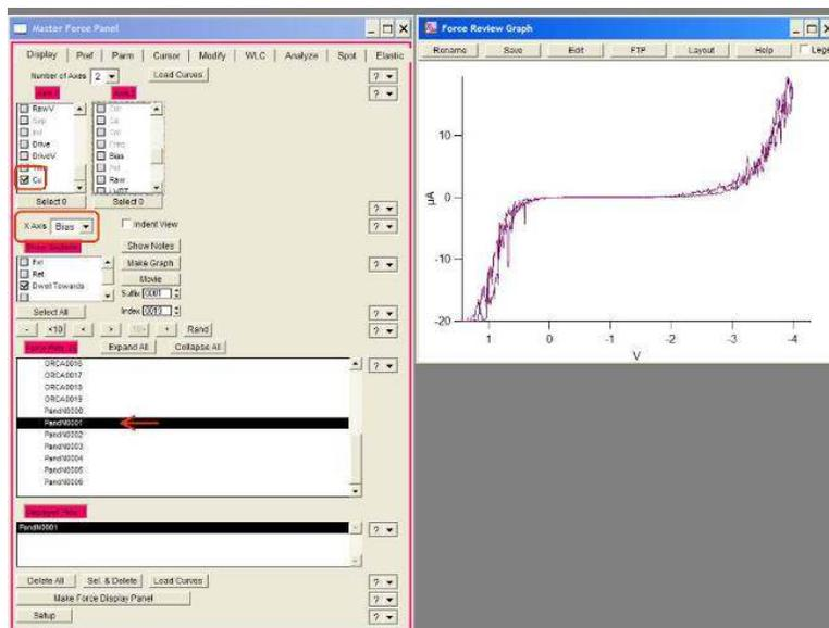
**Figure 9.6.:** Current vs. Bias. To display IV curves, open the force review panel, view current (and current2, if you have a Dual Gain ORCA), set the X Axis to “Bias”, and then select the dwell towards under the sections window. If the graph does not appear, click ‘Make Graph’.
