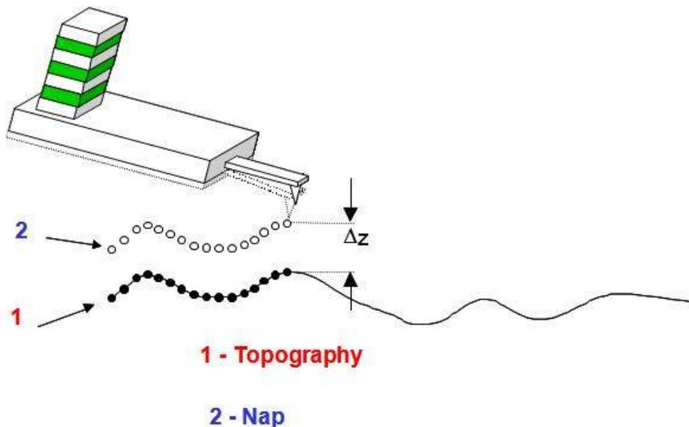
**Figure 11.2.:** Schematic of Nap Mode. For each scan line, the system captures the topography. The system then retraces that topography on the same line to keep a constant distance from the sample surface.
