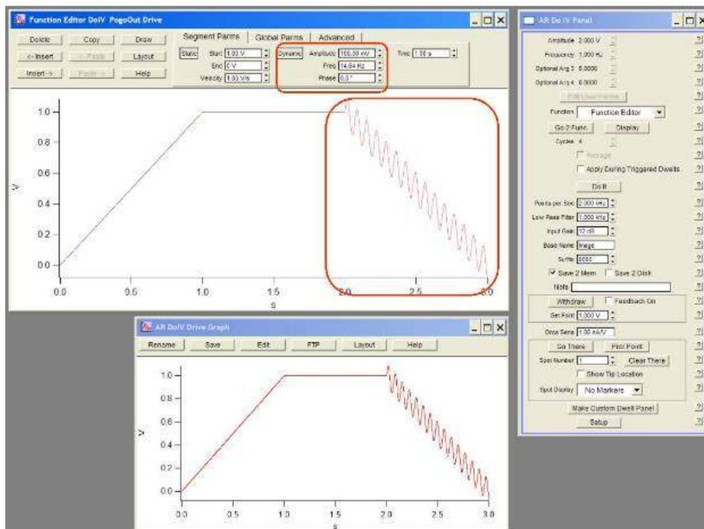
**Figure 9.4.:** The Function Editor can be used to make a variety of drive waves for current measurements. You can insert new segments using the Insert button, select different segments by clicking them., and modify each independently. The Segment Parmns (parameters) tab is shown here.
