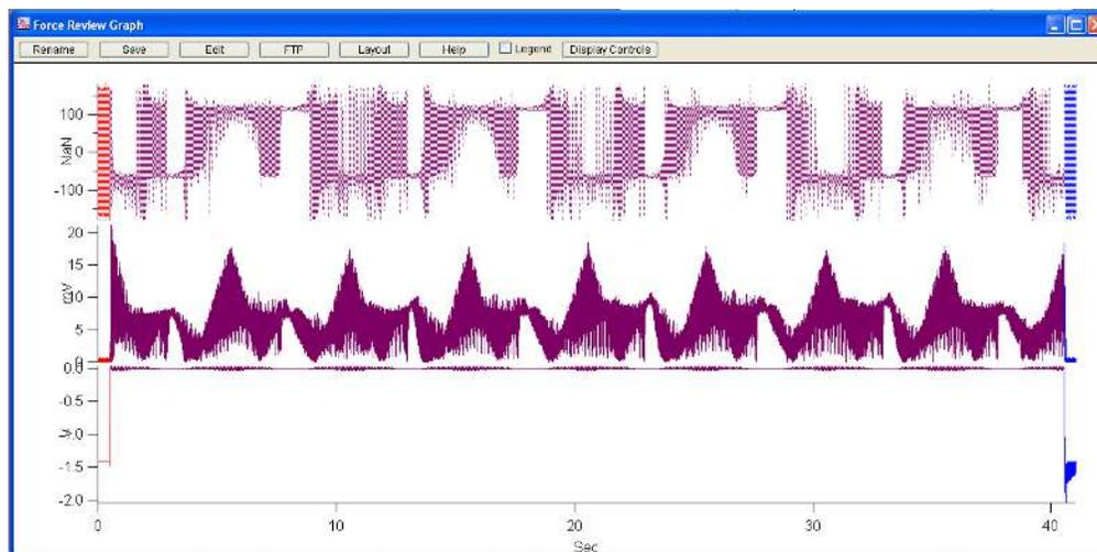
**Figure 8.7.:** The SS-PFM raw data set. The phase1, amp1, and deflection traces for an 8-cycle, 40 second hysteresis loop. The details of the switching are difficult to discern from the time data and need to be processed to produce hysteresis loops.
