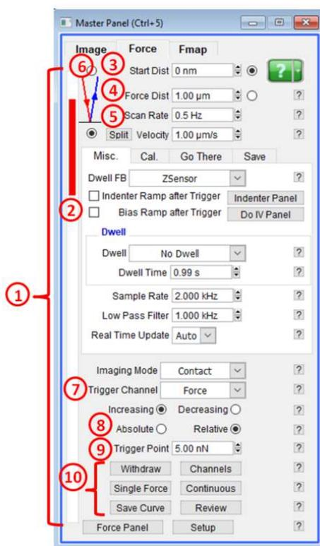
Figure 18.4.: Force tab of the Master Panel.
