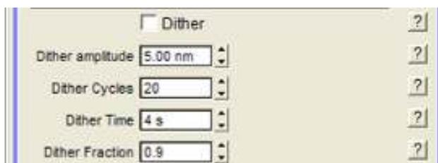
**Figure 9.3.:** The Dither function creates a spiral pattern the probe traces out. This is intended to remove debris or to score the surface in order to get through oxides, thin films, or contamination on the sample surface.
