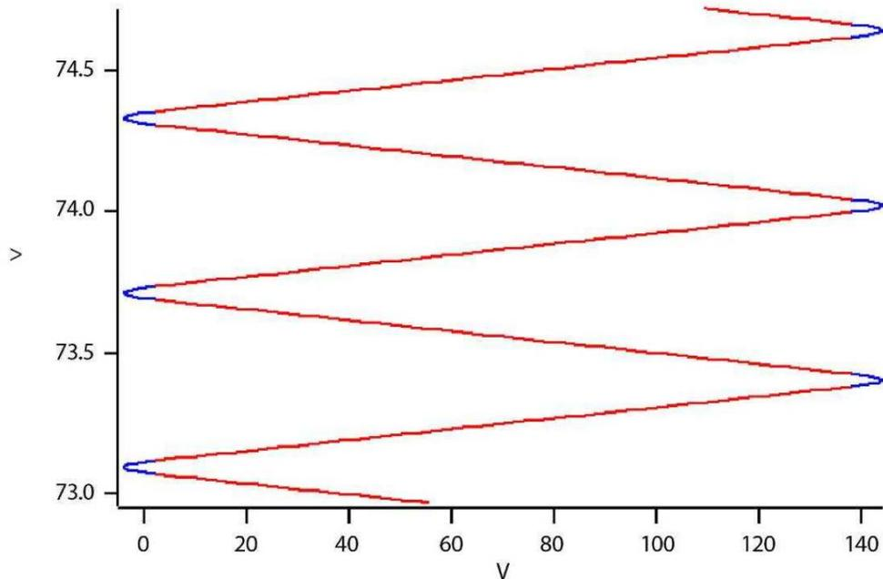
**Figure 23.5.:** X-Y Motion of the Tip across surface in raster imaging. The X-axis is the fast axis drive, while the Y-axis is the slow axis drive. Less than three scan lines are shown to better illustrate the concept. The blue sections denote turn-around regions.
