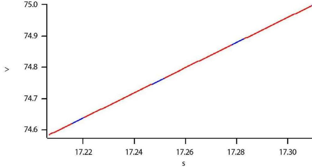
**Figure 23.4.:** Slow Axis of Raster Scan. Y-axis is Y piezo voltage (scan angle 0°); X- axis is time in image above. Axis limits are zoomed in to show the same region as in Figure. The blue sections denote turn-around regions.
