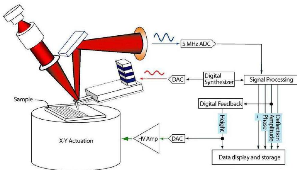
**Figure 5.2.:** Basic diagram of AC mode imaging.
