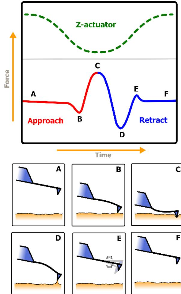
**Figure 17.1.:** Diagram of general Fast Force Map technique. As the Z-actuator changes position sinusoidally versus time, the cantilever force does as well. A, B, C, D, E, and F show discrete points of interest along the curve during the cantilever approach and retraction.
