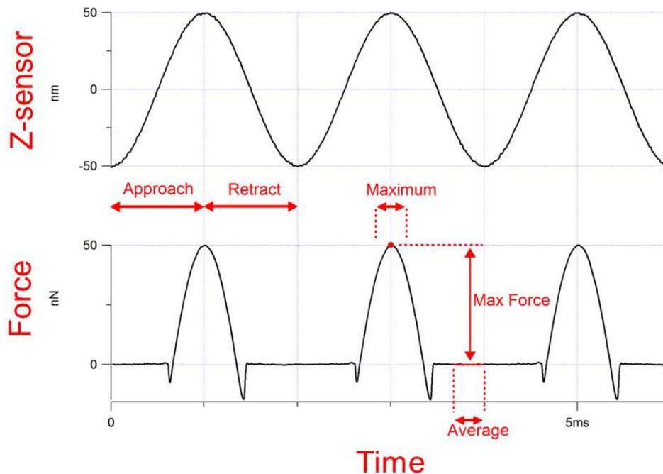
**Figure 17.2.:** Plot of cantilever oscillation measured by the Z-Sensor (excited by driving voltage) (top) and the resulting force (bottom) when the tip is pushing on a hard surface. The “Max Force” arrow indicates how the setpoint force is calculated for each force curve.
