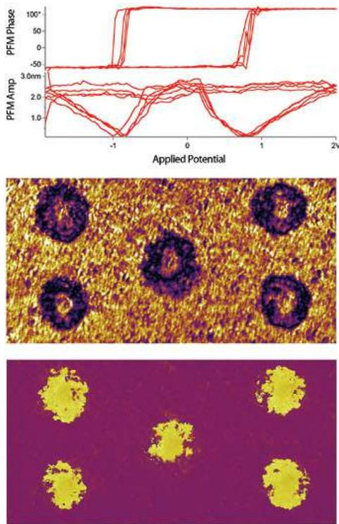
**Figure 6.10.:** Sol gel PZT sample where local hysteresis loops were measured and displayed (representative phase and amplitude loops shown at top). After the switching spectroscopy measurements, the area was imaged, the DART amplitude (middle) and phase (bottom) are shown, 3.5µm scan.
