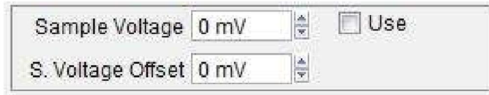
**Figure 9.8.:** Bias and current offsets from the DoIV panel. These can be used to correct for small variations in the outputs of our DACs and the transimpedance current to voltage converter that we use to measure current passing through the sample.
