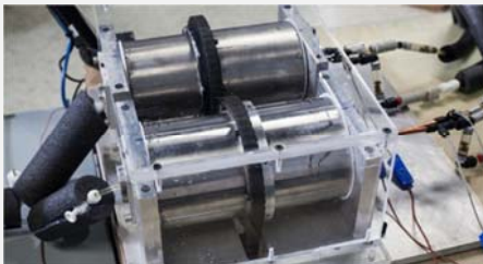
Figure 3.3 GE magnetocaloric device [GE Report, 2014]. Photograph from [GEEK.COM, 2014].
